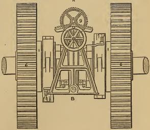
Napier's friction-gear; Fig. 4492 a section through AB; Fig. 4493 a plan; and Fig. 4494 a section through OI, with the friction-straps removed. Fig. 4495 a self-acting friction-brake, which is the basis of the differential clutch.
